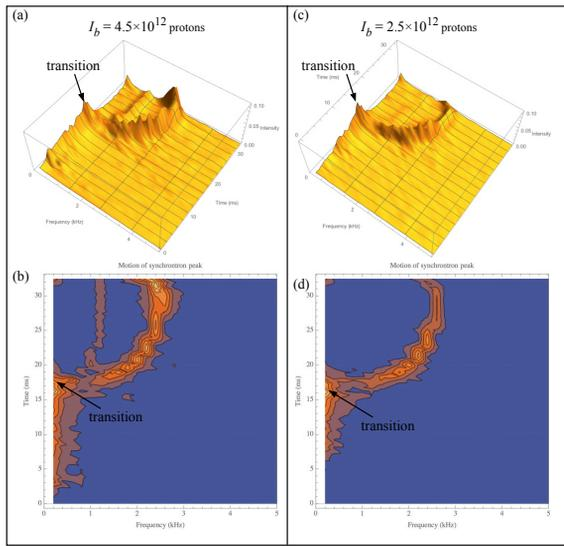
Figure 3: The motion of the intensity normalized  $2\times$  synchrotron peak during the ramp. The quadrupole dampers have been set to a very low gain value (0.1) in these plots.
