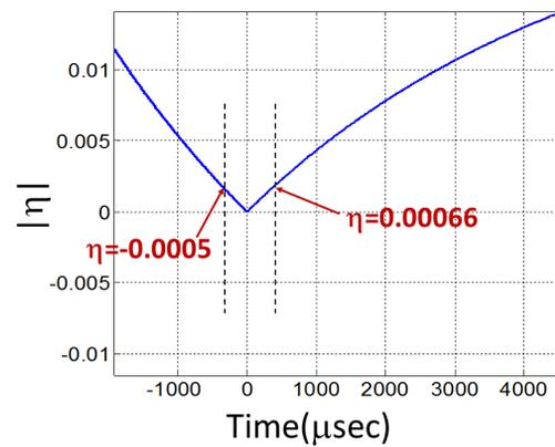
Figure 8: Absolute values of  $\eta$  versus time around transition. The minimum value on the curve corresponds to  $|\eta| = 0$ . The range of  $\eta$  used for the simulations are indicated by the dashed lines.
