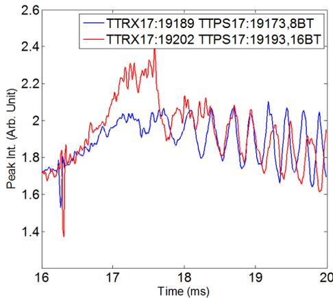
Figure 10: Measured peak intensity oscillations for the optimal settings of transition phase jumps with quad-dampers off for  $2.7 \times 10^{12}$  protons/Booster batch (blue) and  $5.2 \times 10^{12}$  protons/Booster batch (red).
