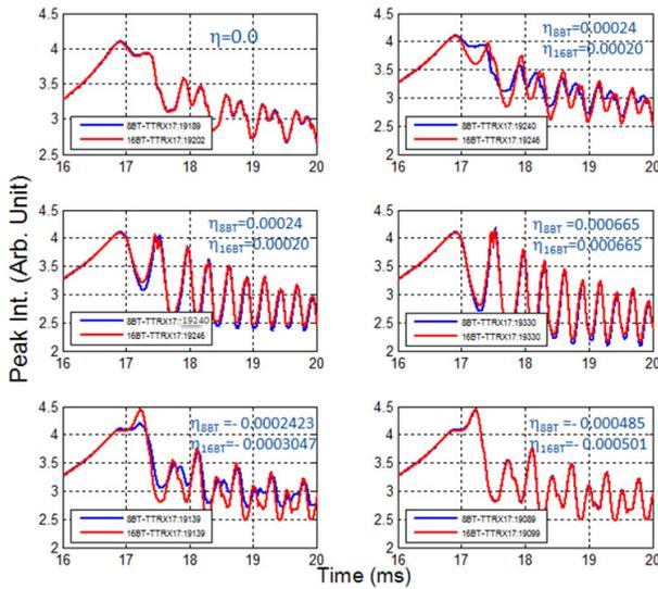
Figure 9: Simulated peak currents as a function of acceleration time for various slip factors around the transition energy. The blue curve is  $3 \times 10^{12}$  and the red curve is  $6 \times 10^{12}$  protons per Booster batch.
