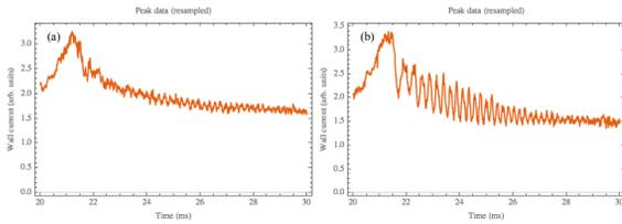
Figure 4: These plots show the envelope of the beam current after processing. Both (a) and (b) were taken with the quadrupole dampers on and beam current  $\sim 4.5 \times 10^{12}$  protons.
