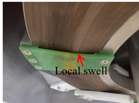
Figure 10: Local damage of type B MA core.
