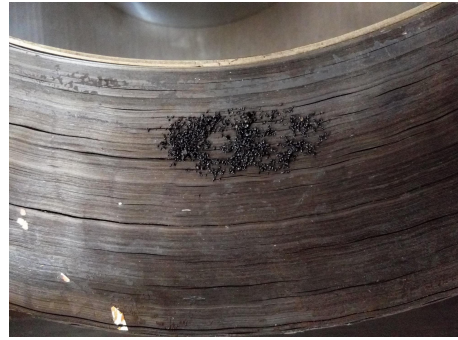
Figure 8: Local damage of type A MA core.
