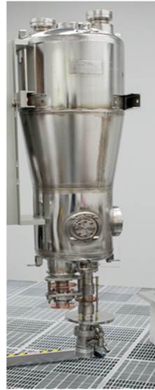
Figure 3: 72.75 MHz quarter wave resonator.
