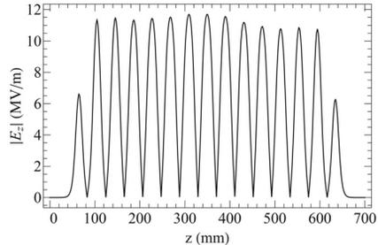
Figure 4. CST model for the 15-gap CH cavity (top) and accelerating electrical field along the cavity (bottom).
