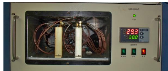
Figure 4: Temperature stabilizing chamber.
