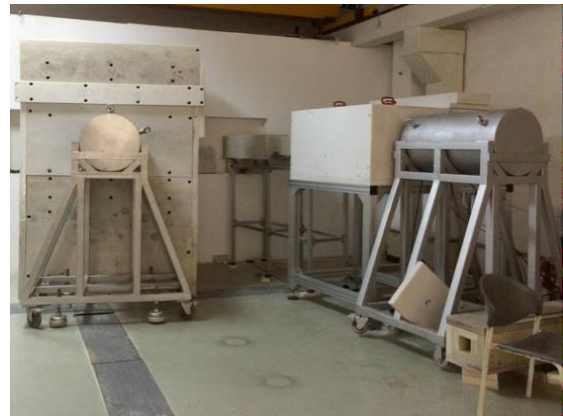
Figure 8: The neutron imaging line (left) and neutron beam test line (right).
