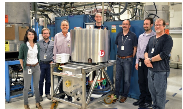
L-3 Communications Electron Devices' L6200 1.2 MW, 704 MHz Multi-Beam IOT for ESS
