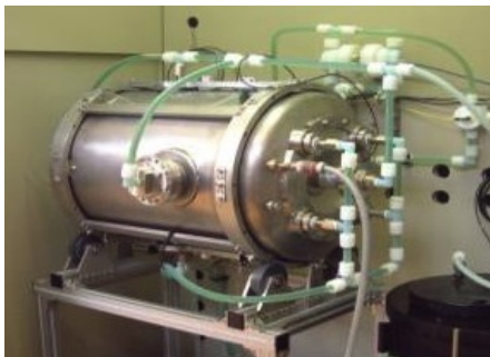
Prototype cavity at IPNO set up for surface treatment
