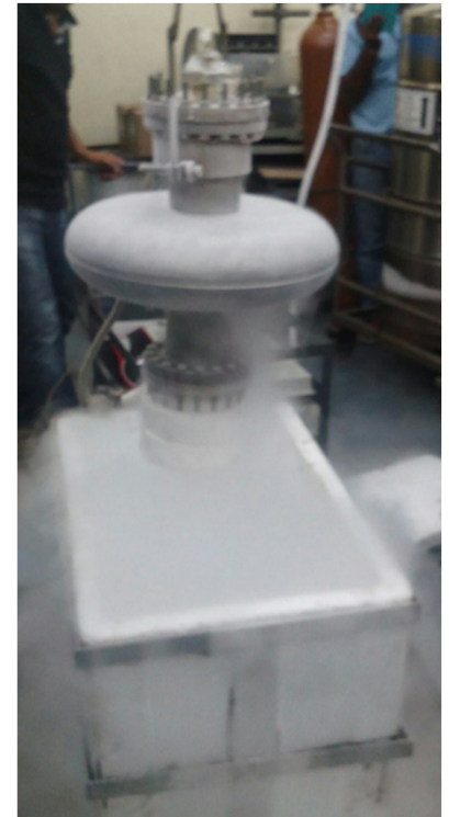
Vacuum leak rate checking of single cell cavity at LN 2 temperature
