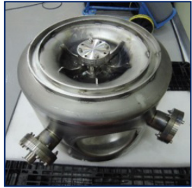
SSR SC Cavity and its Cryomodule
