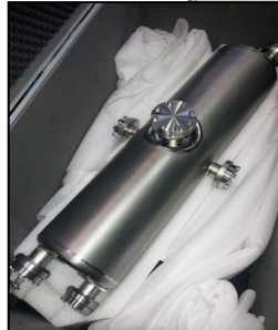
HWR SC Cavity & its Cryomodule
