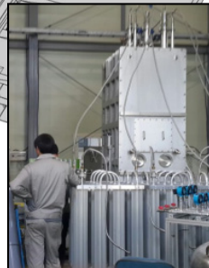
HWR SC Cavity & its Cryomodule
