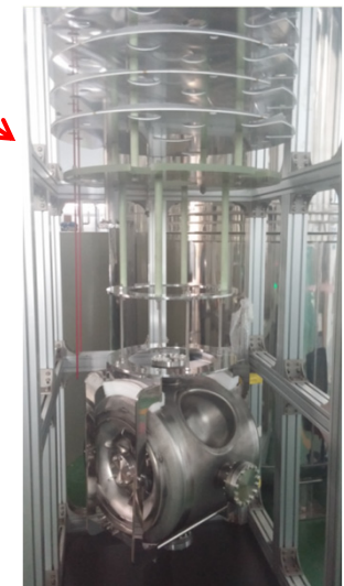
Vertical cavity test
