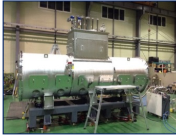
SSR SC Cavity and its Cryomodule
