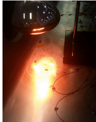
Curing of epoxy glue
