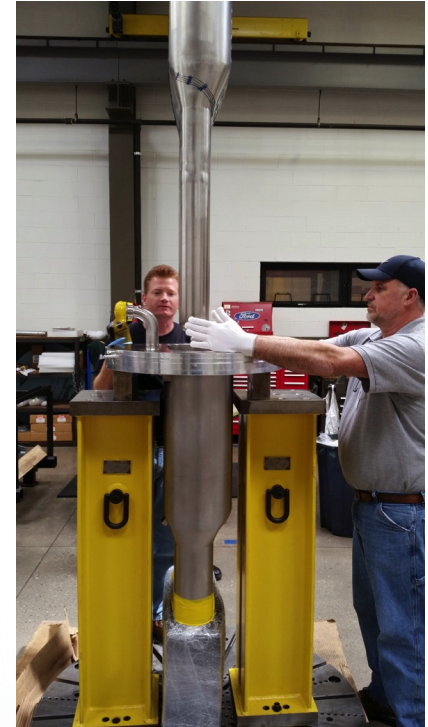
Vessel being inserted into the water-cooled shroud.
