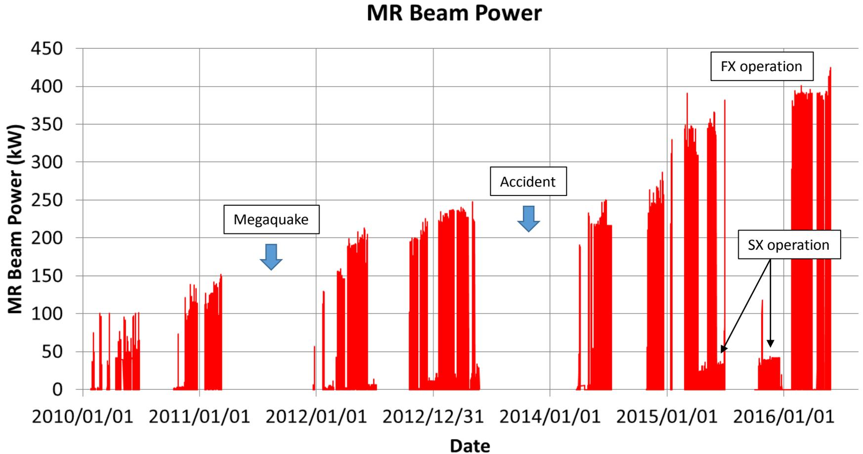
The MR beam power has been increasing. Now we have  $2.15 \times 10^{14}$  protons per 2.48 s pulse. It is important to [handle and localize beam losses](#) for maintenance and machine protection.
