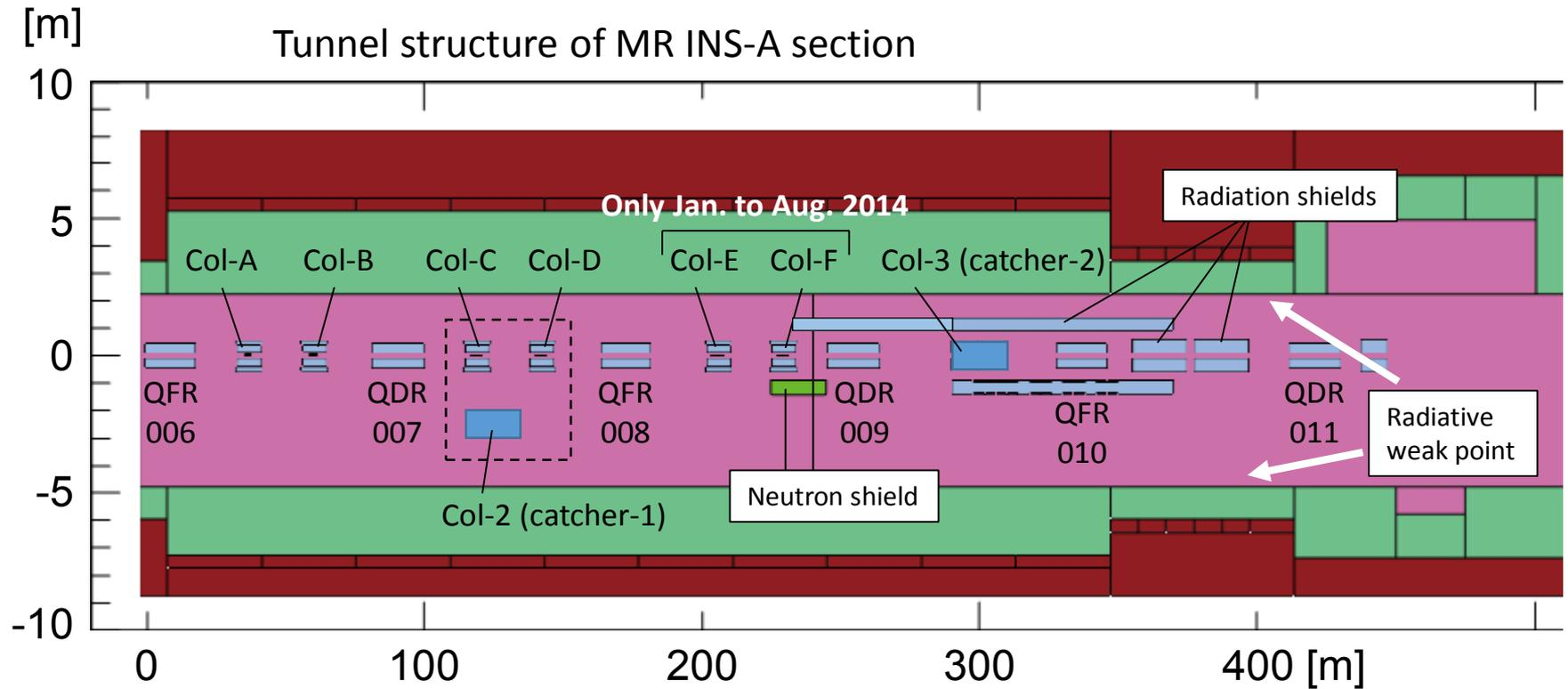
History of the collimator layout with the schematic view of accelerator tunnel.
