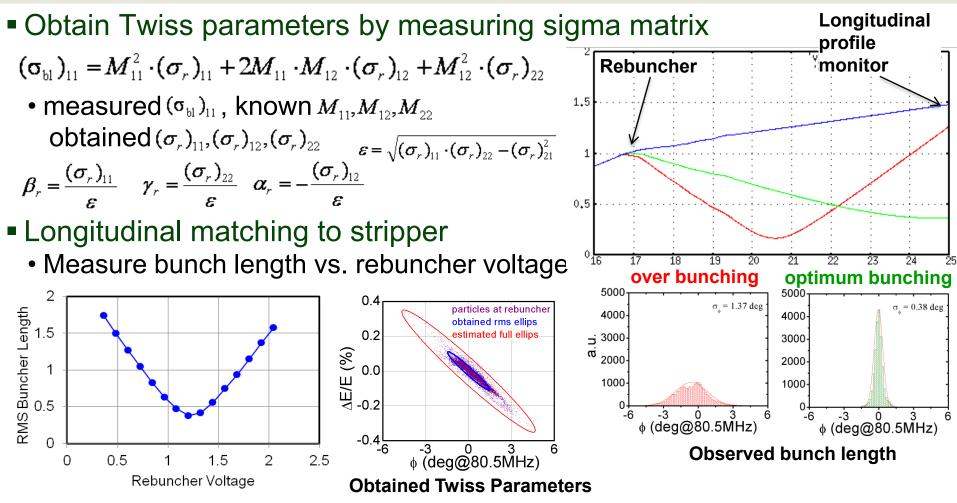
Same method applies transverse matching by quad/solenoid scanning
