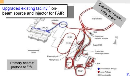
Accelerator Components & Key Characteristics Ring/Device Beam Intensity Energy SIS 100 (100Tm)  $4x10^{13}$ protons 30 GeV 238U 1 GeV/u 5x10<sup>11</sup> (intensity factor 100 over present) <sup>40</sup>Ar 45 GeV/u 2x109 SIS 300 (300Tm) 238[] 2x10<sup>10</sup> 34 GeV/u CR/RESR/NESR ion and antiproton storage and experiment rings **HESR** antiprotons 14 GeV ~1011 <109 Super-FRS rare isotope beams 1 GeV/u
