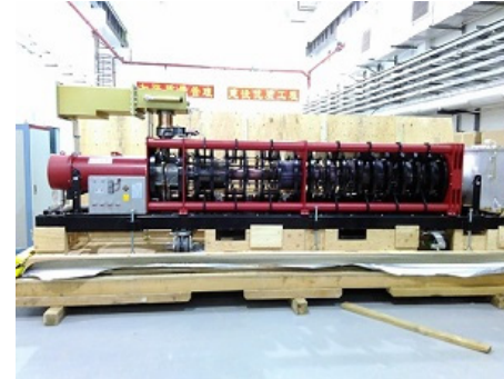
IGBT solid state switch modulator
