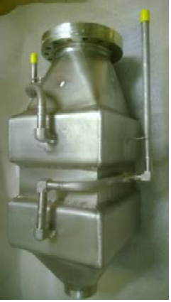
He/He Heat exchanger (Superfluid helium production)
