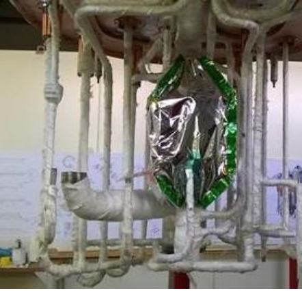
He/He Heat exchanger (Superfluid helium production)
