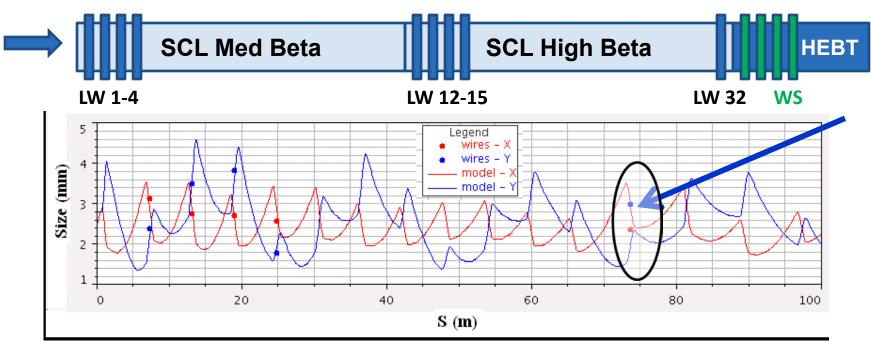
"Figure 7 shows one of the general cases: fit beam size for the first 4 laser wires with the online model, and then compare model prediction against measurement at the 5th wire – they do not agree at all."
