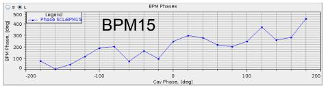
An example of Cav01a scan. We cannot go further BPM07 with the step size 20<sup>0</sup>
