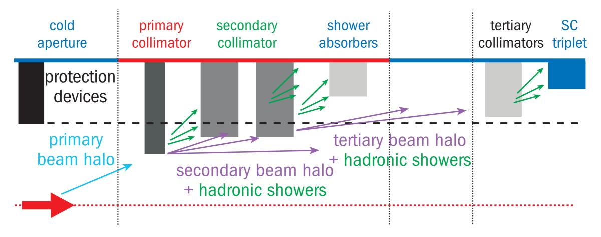
Three-stage cleaning in two warm insertions: betatron (IR7) and offmomentum (IR3); local "tertiary" collimators at inner triplet.
