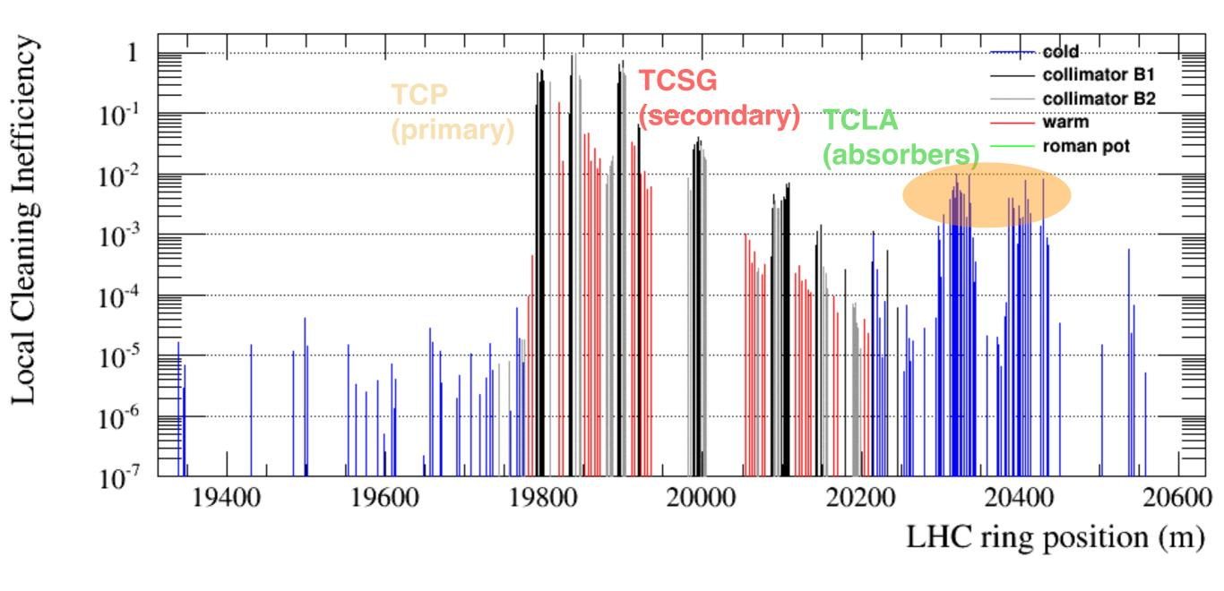
Betratron cleaning of ion beams limited by ion fragments: a few 0.01, i.e. 100 times worst than for protons.
