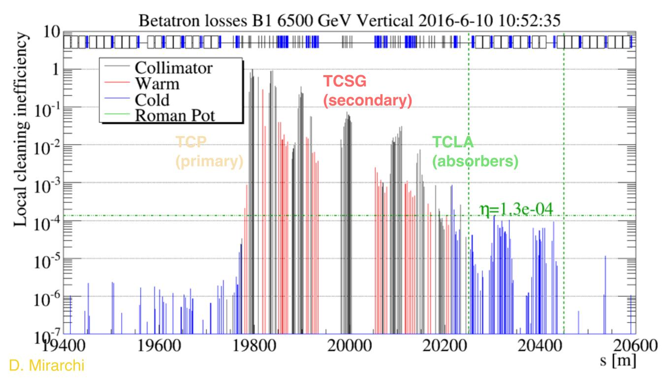
Limiting locations for cleaning: dispersion suppressors around IR7
