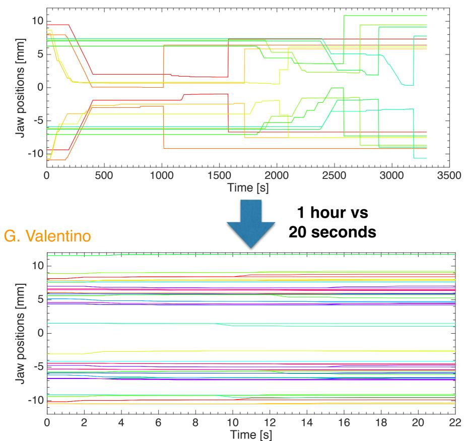
Standard method: collimators closed until each jaw touches the beam halo. One collimator per beam at a time.
