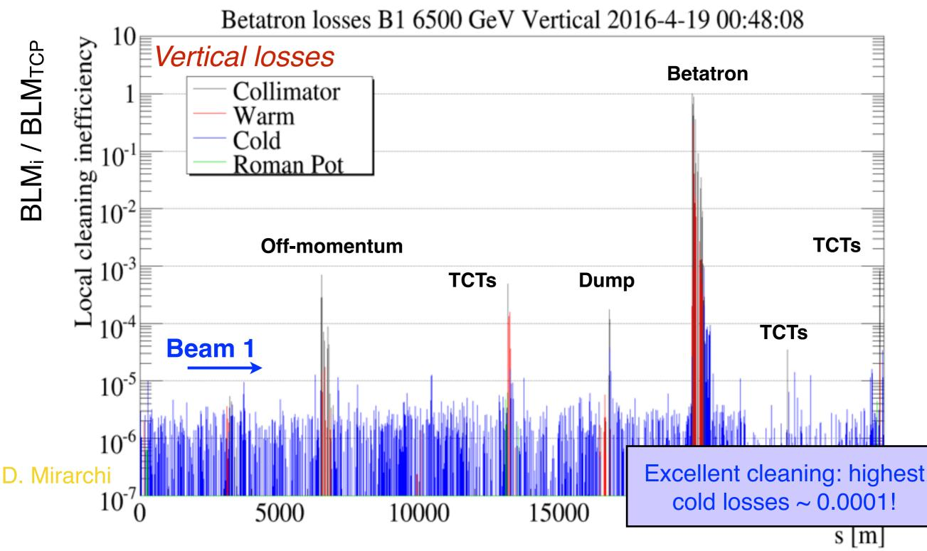
System validation through controlled excitations of transverse beam losses (triggered by transverse damper).
