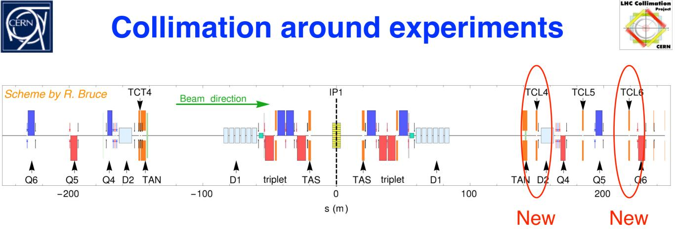
In preparation for the **high-luminosity** operation at **6.5 TeV**, improved the **physics debris collimation** downstream of ATLAS an CMS:
